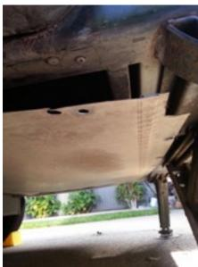
When I got home I searched Airforums and discovered that ours was not an isolated incident. Belly pans can work their way loose from the rivets by long-term use for the following reasons: Constant flexing from harsh roadways, heavy winds, and stresses caused from load-leveling hitches adjusted improperly, which creates stress on the rear portion of our trailers.
