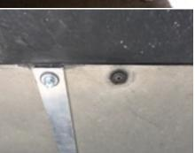
With the help of our fellow member and good friend Rick, we made the repairs by cutting strips of aluminum and using "Self-Drilling 12x1" hex with neoprene washers" available from Lowe's Home Center. On the jack, it was only a matter of replacing the mission jack bolt and tightening it up.
